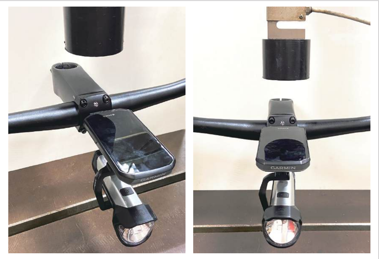
Bracket fatigue test method: Impact 150kg/f at the stem/handle-bar. load of 1,000 grams at the extension arm and run for 100,000 times.
